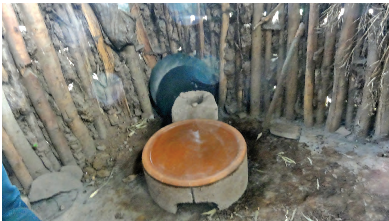
Figure 13.3 Mirt stove just installed at farmer's house kitchen. Photo by Zenebe Gebreegziabher.
